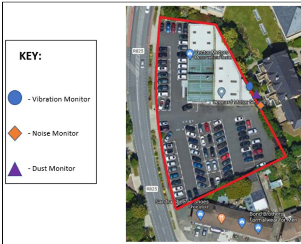
Figure 7.3 Proposed construction stage air quality, noise and vibration monitoring locations if required
