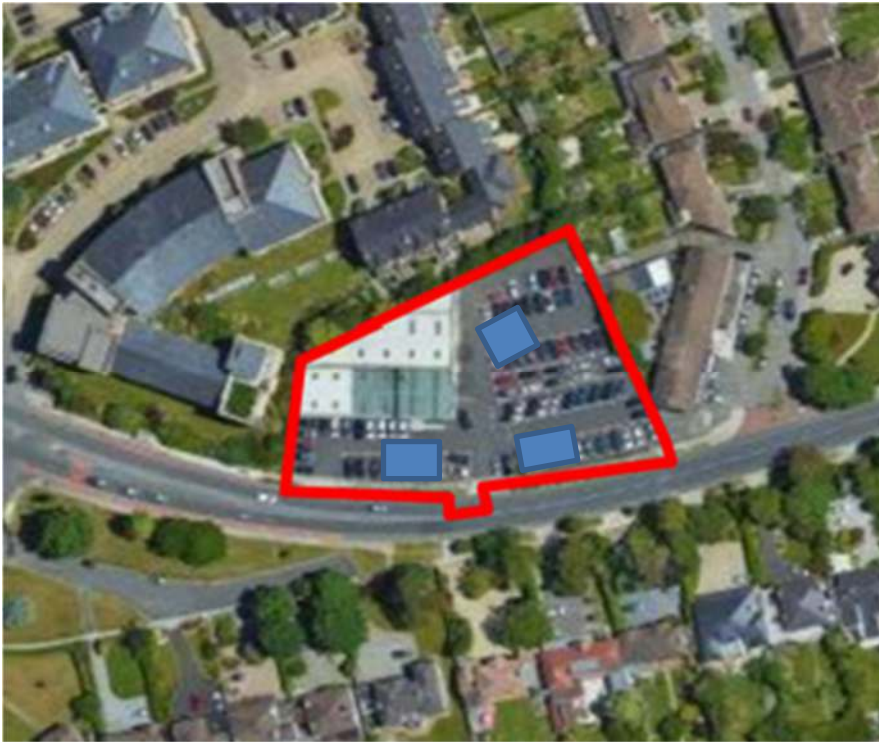
Figure 5.1 Potential site construction compound locations (illustrated by blue boxes)
